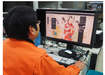
▲[Photo 1] Image data is broken down into four CMYK colors. Color decomposition is performed while assuming the color tones of the ceramic board, and the original data for the transfer paper is created.
