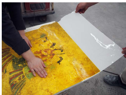
▲[Photo 3] The transfer paper is pasted onto a ceramic board that reproduces only the unevenness of the surface. The paper is carefully attached to the ceramic board so that the unevenness of the plate and the transfer paper do not shift, and so that the paper does not tear due to the unevenness of the plate.
